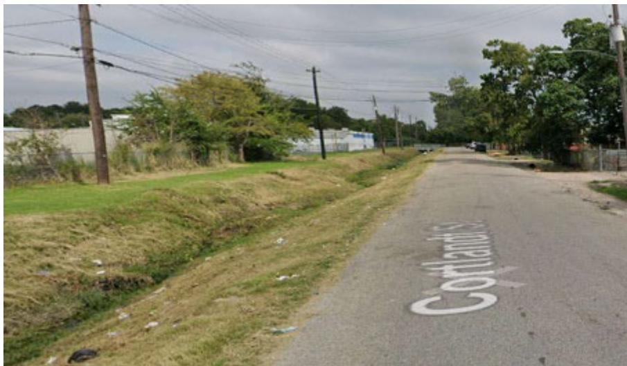
The existing channel does not contain the 10-yr storm event within the banks. Future HCFCD improvements are to upgrade the channel to a 12'x10' RCB from I-45 to Little White Oak Bayou.
