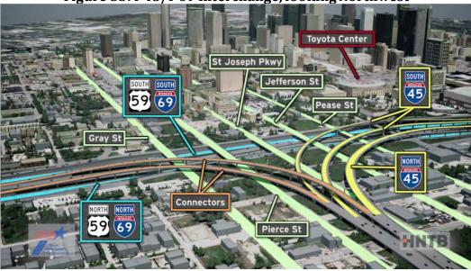
The configuration resulting from the removal of the elevated freeways and replacing with depressed freeways, would enhance the connectivity between downtown and the East Downtown Houston (EaDo) neighborhood. This depressed area would allow for the installation of a decked park similar to the Klyde Warren Park in Dallas, TX, as depicted in **Figure 54**.
