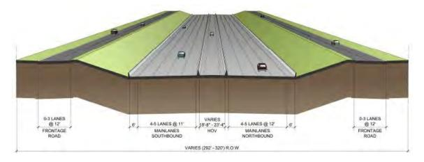
Figure 4: I-45 Existing Typical Section from I-10 to Allen Parkway
