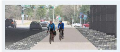
Artistic rendering as example of brick pavers and concrete path along an off street pedestrian and bike facility under the highway.
