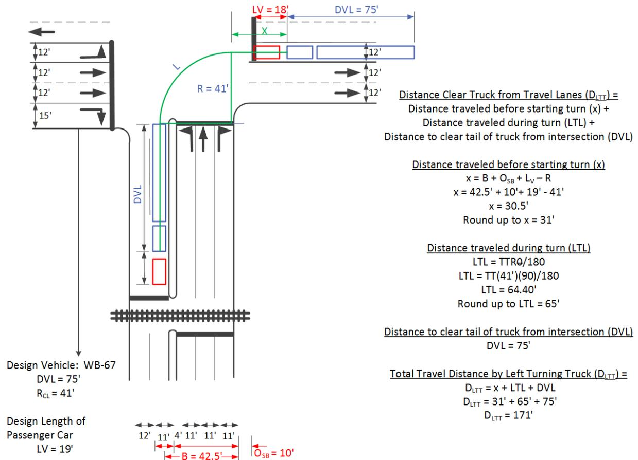
Figure 2. Sample calculation of the distance required to clear left-turning truck from travel lanes on track clearance phase.
