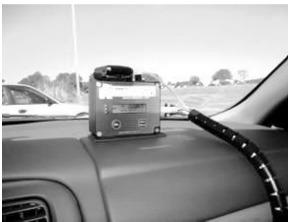
Figure 5-4. Equipment setup in test vehicle-GPS positioning.
