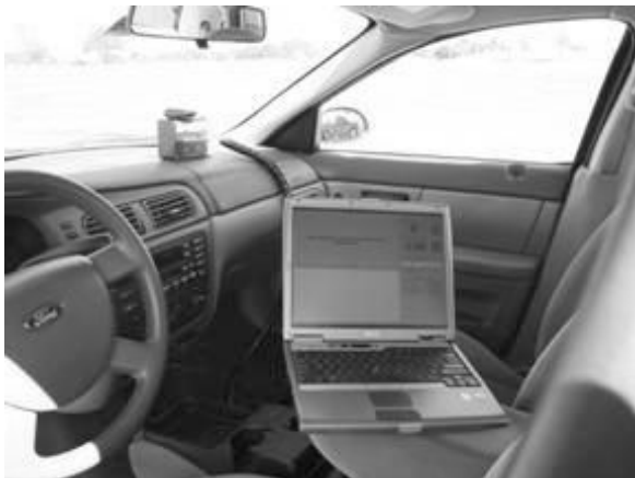
Figure 5-3. Equipment setup in test vehicle-laptop positioning.
