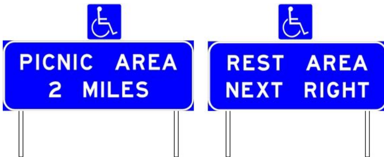
Figure 7-18. ADA Accessibility plaques (D9-6) attached to advance picnic and rest area signs for divided highways and freeways
