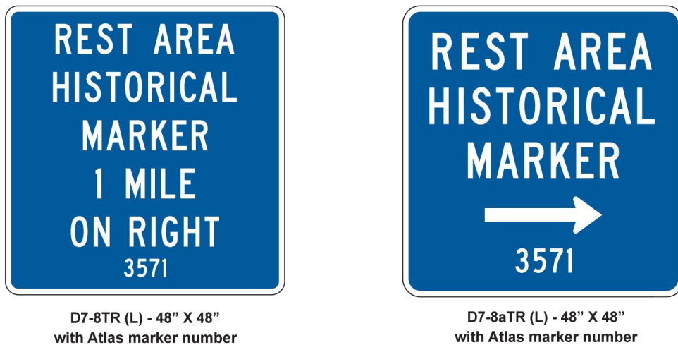
Figure 7-13. Advance and directional rest area historical marker guide signs with Atlas marker numbers. Colors: legend - white (retroreflective); background - blue (retroreflective)
