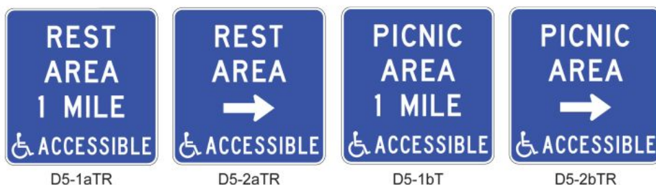
Figure 7-19. Advance and directional rest area signs (D5 series) for conventional highways showing ADA accessible message
