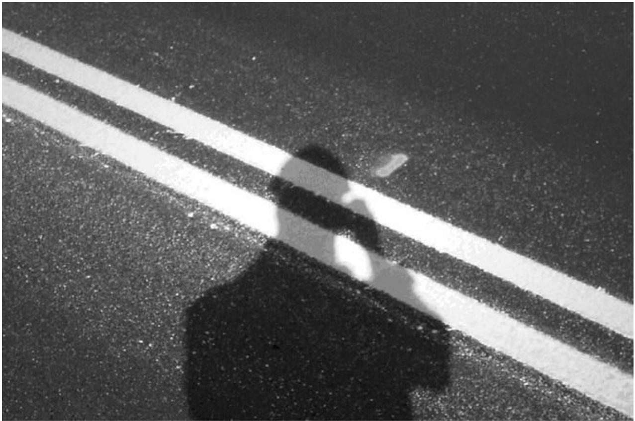
Figure 3-5. Sun-over-shoulder test from Test Method Tex-828-B.
