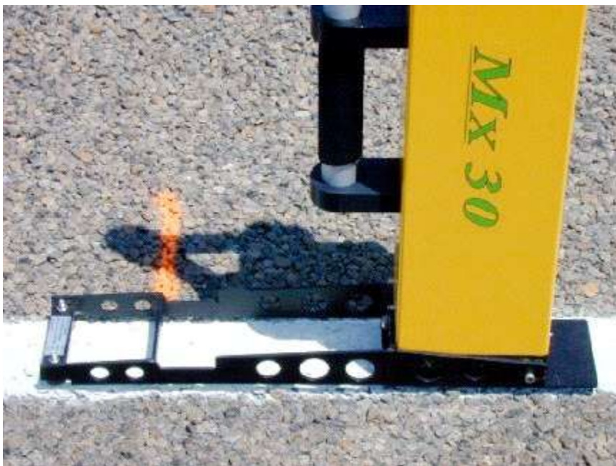
Figure 3-6. Handheld instrument prepared for retroreflectivity measurement.
