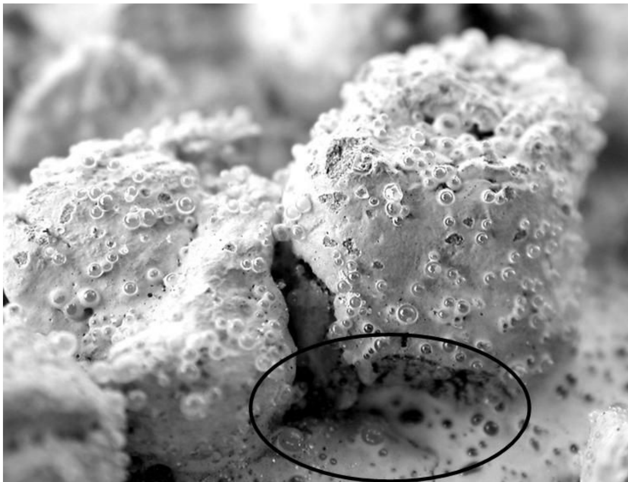
Figure 2-2. Beads falling between aggregates.
