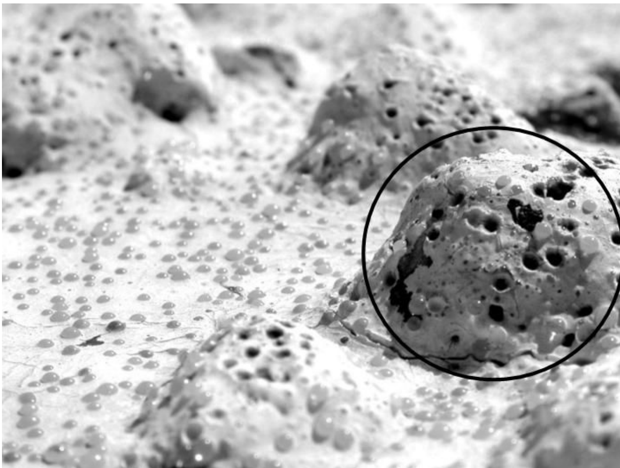
Figure 2-5. Poor bead retention on top of aggregates.
