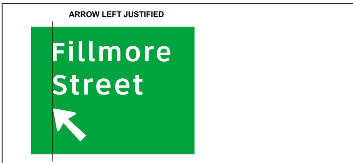
Figure 4-40. Arrow placement with roadway designation on the second line of copy.
