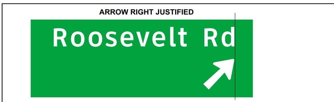
Figure 4-35. Preferred arrow placement with one word message.
