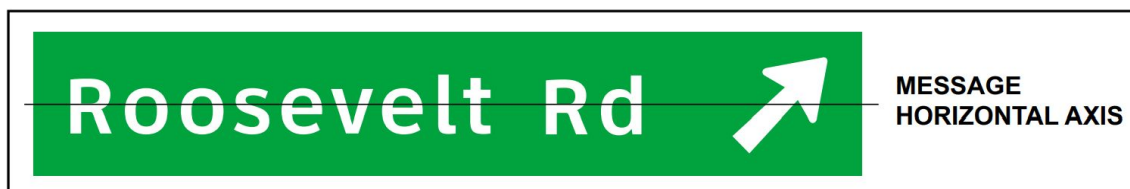
Figure 4-37. Arrow placement with word message on the same line of copy.
