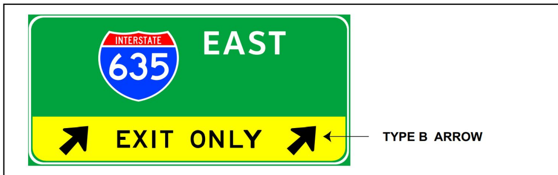
Figure 4-6. Type B arrows used on an Exit Only panel.
