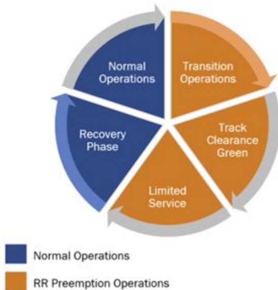
Figure 6–14. Generic Railroad Preemption Sequence
