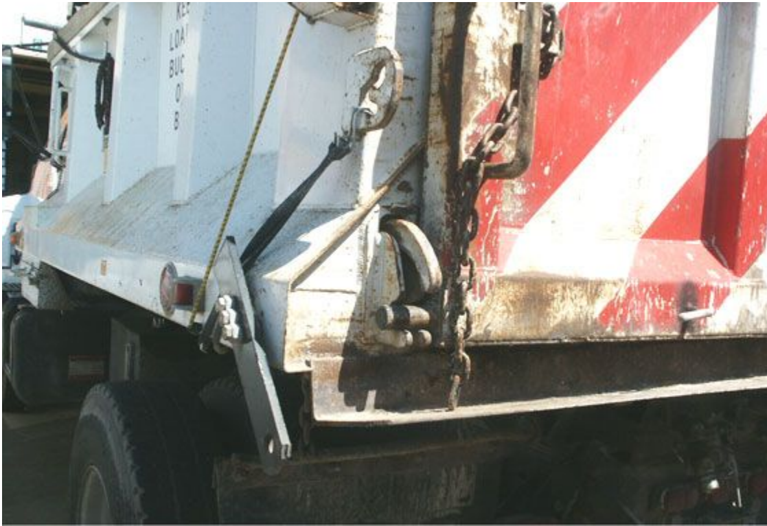
Figure 7-39. Latch on Tailgate of Haul Truck.
