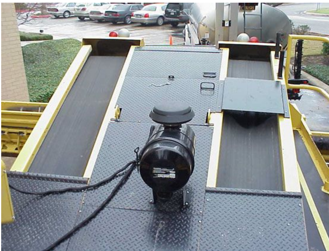
Figure 7-30. Belt Conveyors on Aggregate Spreader.
