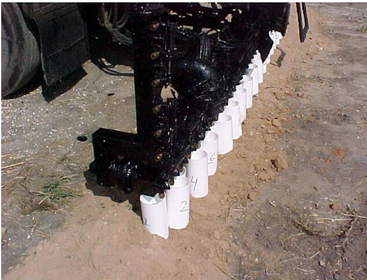
Figure 7-21. Calibration of Asphalt Distributor Spray Bar.
