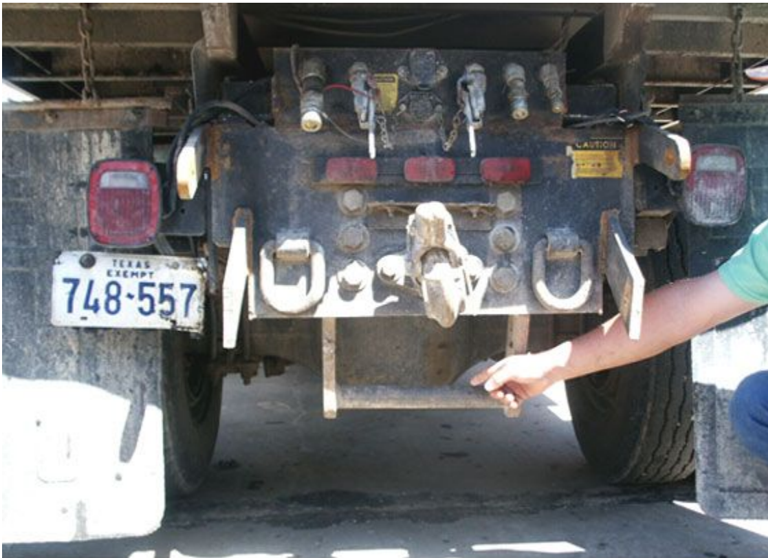
Figure 7-40. Truck Hitch to Connect to Aggregate Spreader.
