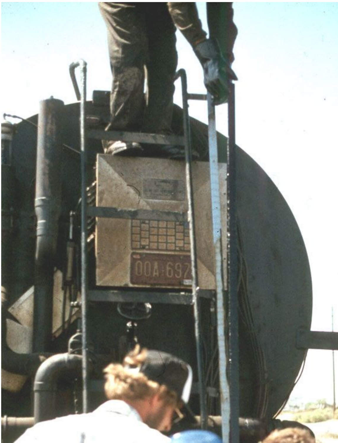
Figure 7-25. Strap Stick Used to Measure Quantity of Asphalt in Distributor Tank.
