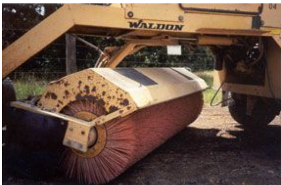
Figure 7-2. Bristle Brush on Rotary Broom.
