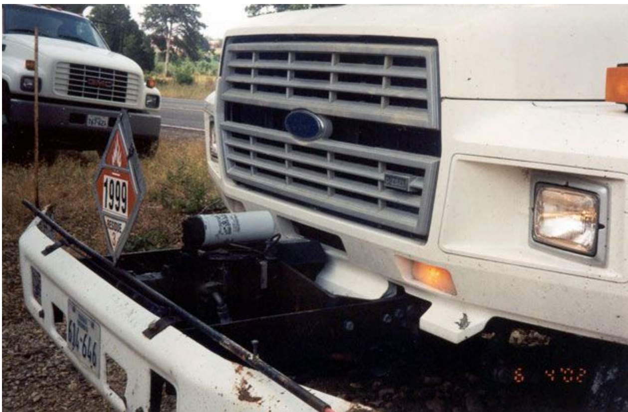
Figure 7-8. Hydrostatic Distributor Located at Front of Truck.
