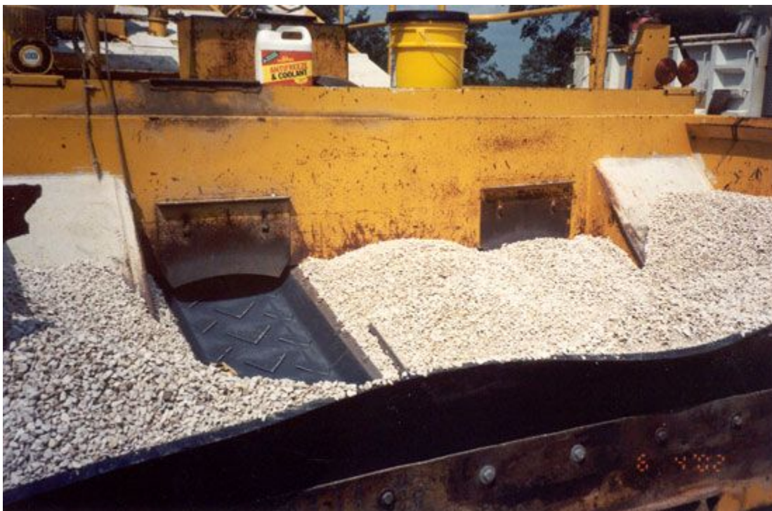
Figure 7-29. Receiving Hopper of Aggregate Spreader.
