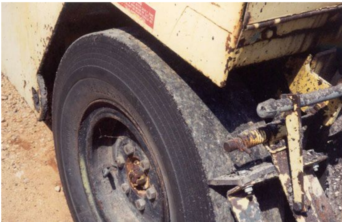
Figure 7-45. Smooth-Surfaced Pneumatic Tire.
