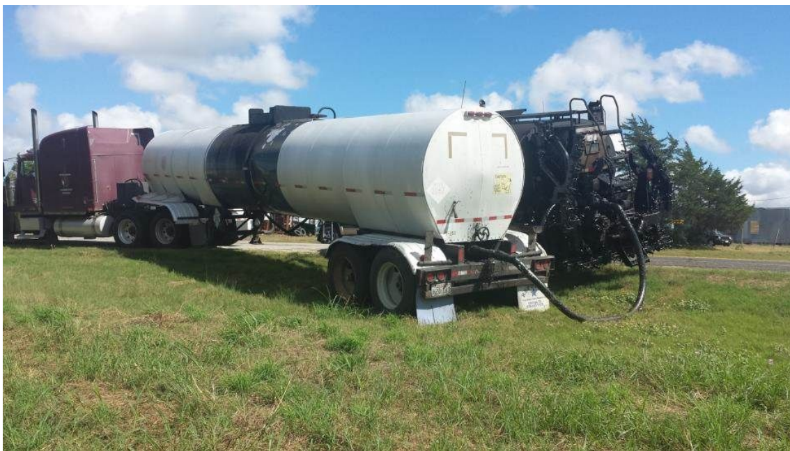
Figure 8-5. Transferring Asphalt from Transporter to Distributor.
