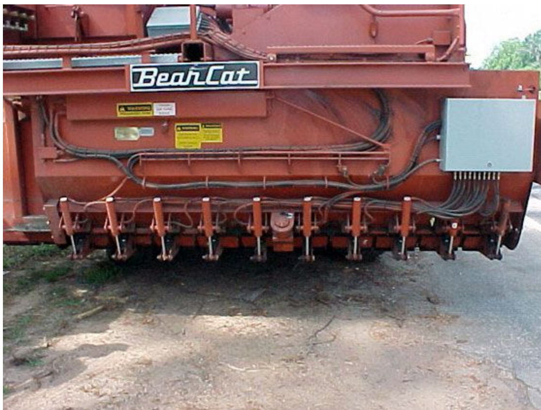
Figure 7-32. Discharge Gates on Aggregate Spreader.
