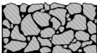
Fig. 3.5a Gap-graded (Performance-Designed or SMA) mix
