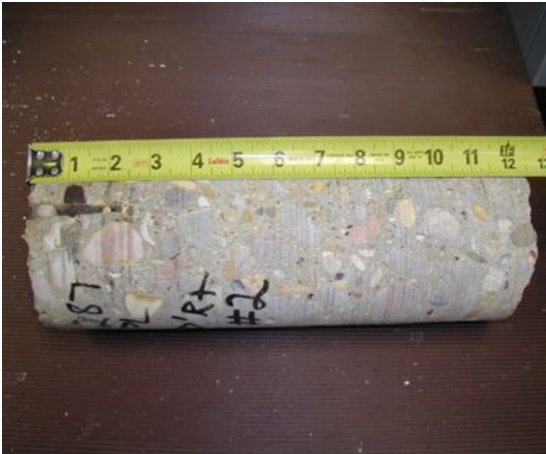
Figure 9-74. Crack was not induced due to shallower saw-cut depth than required.
