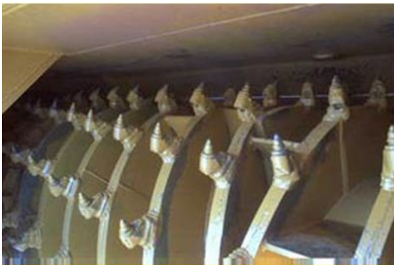
Figure 10-16. Teeth of the Rotomill.
