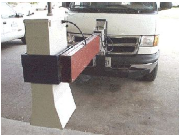
Figure 4-8. Air-coupled Ground Penetrating Radar (GPR).
