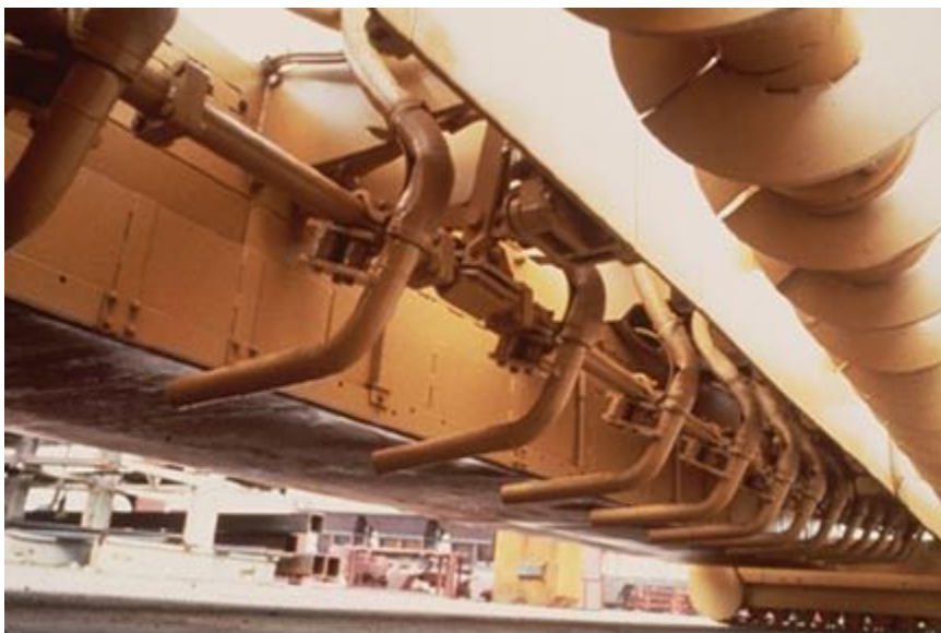
Figure 9-45. Underside of slip-form paver.
