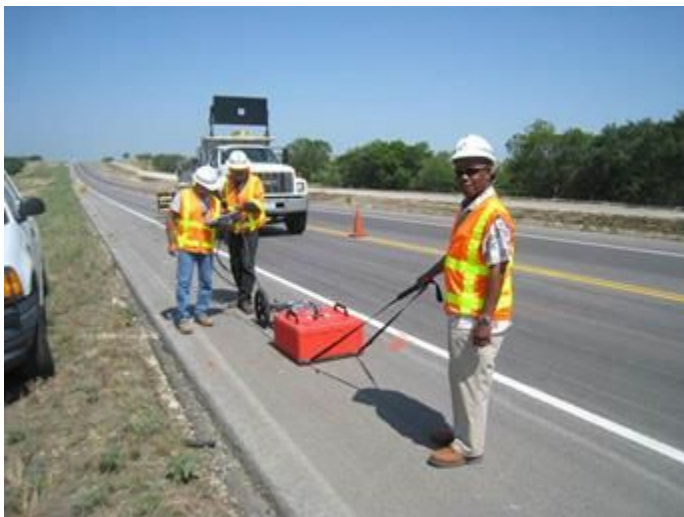
Figure 4-10. 200 MHz Ground-coupled Penetrating Radar.
