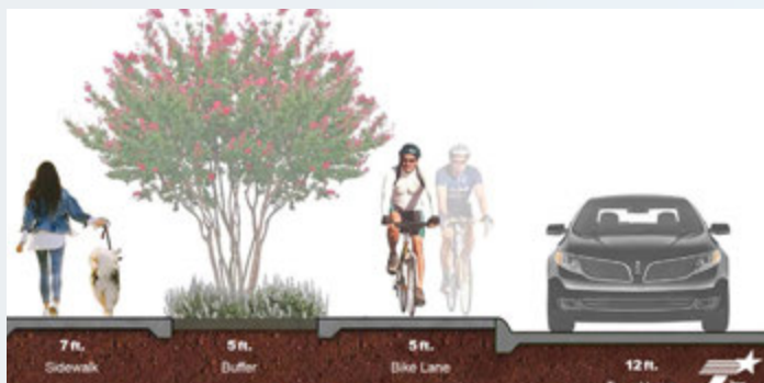
Artistic rendering depicts one-way elevated bike lane behind the curb with buffer between pedestrians and bikes to allow for tree plantings. Illustration not drawn to scale and is subject to change.
