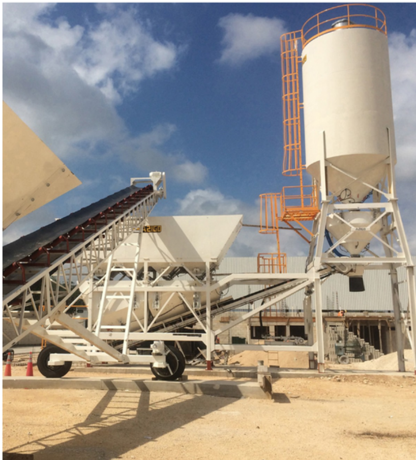
Pictured above is a temporary wet batch concrete plant.
