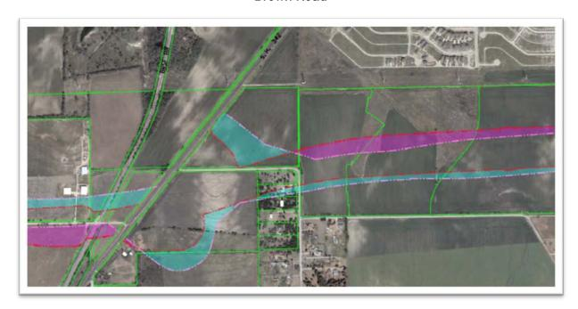
Exhibit 4: Loop 9 shift at SH 342 by converting loop ramps to jug handles
