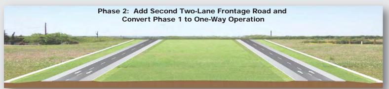
As traffic warrants and funding becomes available, PHASE 2 would involve the construction of the second two-lane frontage road and the conversion of the two-way frontage road built in Phase 1 to a one-way operation. This frontage road facility would include:
