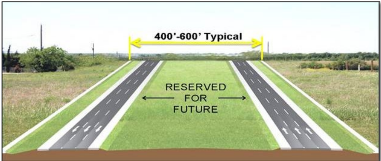
Figure 1-1: Segment A, Phase II Construction of One-Way Frontage Roads
