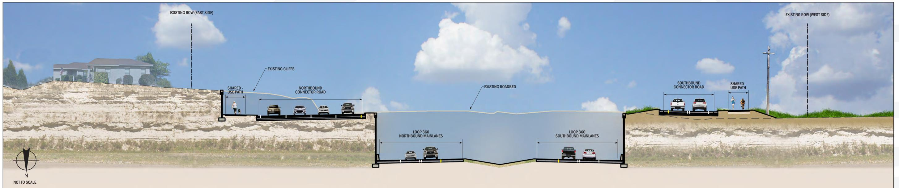
The new configuration of Loop 360 just south of Westlake Drive will include free-flow underpass lanes and connector roads with through and turn lanes to Westlake Drive.
