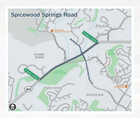
This project includes removing the traffic signal on the mainlanes at Loop 360 and Spicewood Springs Road (E)/Bluffstone Drive and adding an overpass. The project also includes removing the signal at Loop 360 and Spicewood Springs Road (W), as well as adding bicycle and pedestrian improvements within the project limits.
