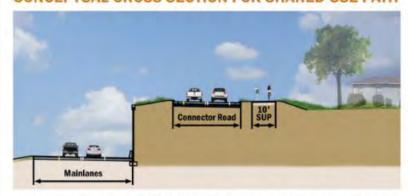
10 foot shared-use path with 5 foot buffer as right of way allows
