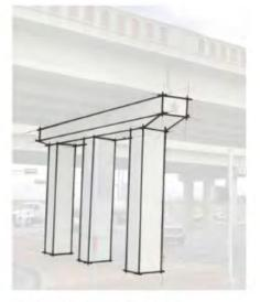
BENT CAP Standard Sloped
