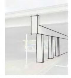
BENT CAP Standard Rectangular with Ear Wall
