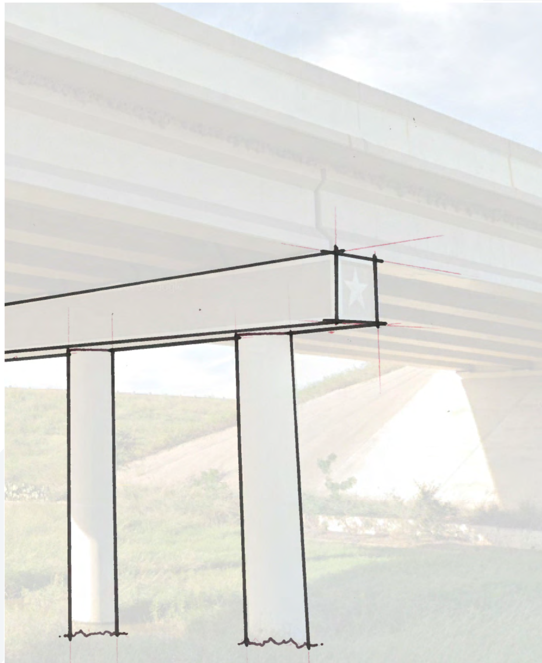
BENT CAP Standard Rectangular COLUMNS Round
