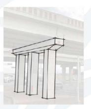
BENT CAP Standard Sloped **COLUMNS** Square
