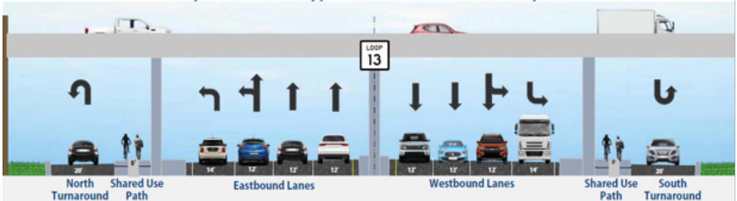
Proposed SL 13 Typical Section at I-37 Overpass
