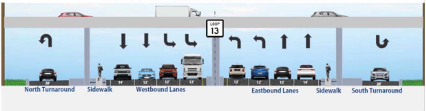
Proposed SL 13 Typical Section at I-37 Overpass
