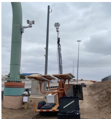
Figure 2. Silent sentinel camera and solar trailer.
