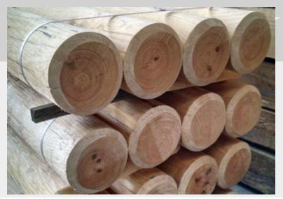
Furnish treated poles in accordance with AWPA to the minimum net retention and penetration of preservative treatment in accordance with Table 1.
