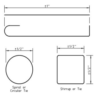
Figure 1 Fabrication Tolerances for Bars
