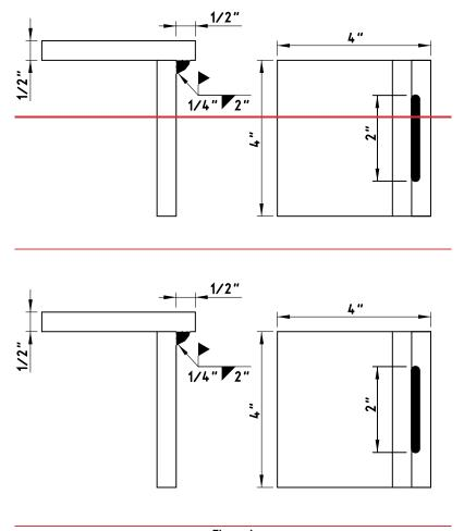
Figure 1 Miscellaneous Qualification—Fillet Weld Break Specimen
