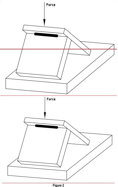
Miscellaneous Qualification—Method of Rupturing Specimen
