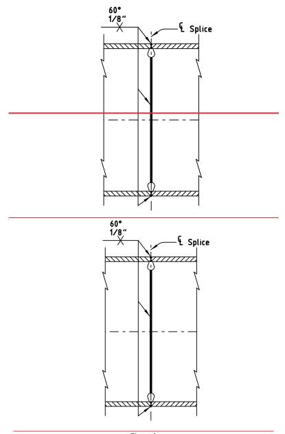
Figure 3 Girder Splice Details
