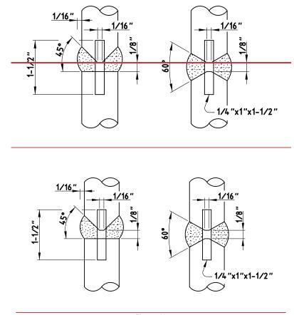
Figure 10 Double Bevel <u>and Double</u> V-Groove <del>WeldWelds</del> in Vertical Position
