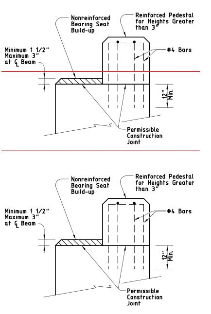
Figure 1 Section <del>through<u>Through</u> Bearing Seat Buildups</del>
