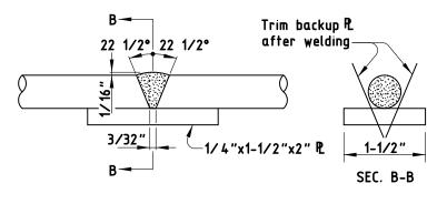
Figure 8 Single Bevel V-Groove Weld in Horizontal Position
