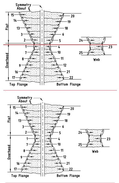
Figure 6 Welding Sequence for Splices for Material up to 50,000-psi Yield Strength<del>.</del>
