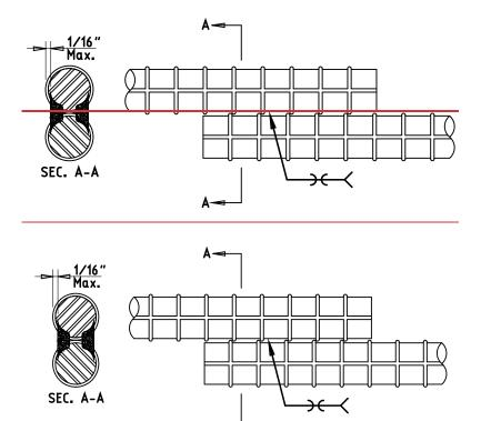
Figure 7 Direct Lap Joint with Bars in Contact
