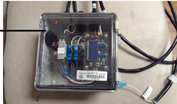
This "sensor kit" interfaces between operations sensors and inputs on the existing fleet tracking system.
