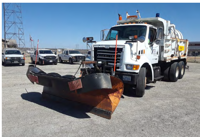
Brine sprayer and plow equipped with operations sensing capabilities.
