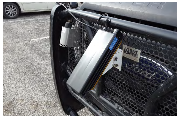
The surface condition sensor monitors roadway surface for temperature and wetness, reporting readings in a web-based environment.
