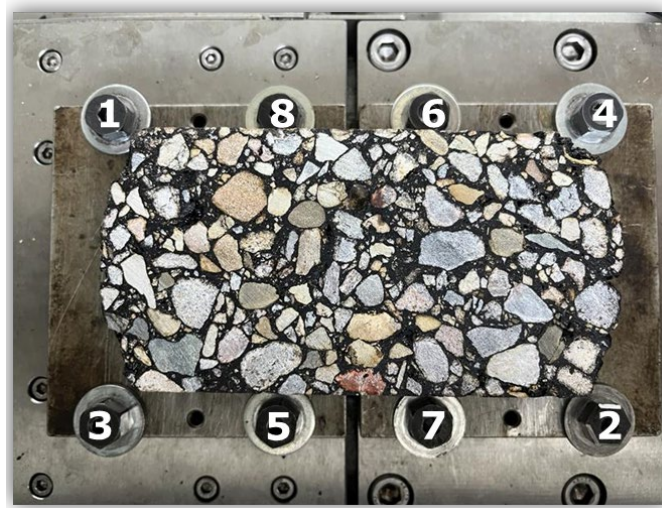
Figure 5.4 – Recommended Bolt Tightening Pattern
