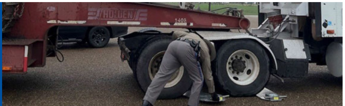
Trooper Using Portable Scales During a CMV Inspection.
