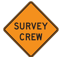
CW21-6 SURVEY CREW
