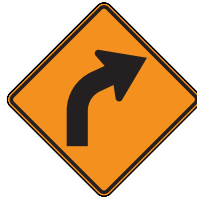
CW1-2R Horizontal Alignment - Curve
