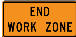
G20-2bT END WORK ZONE
