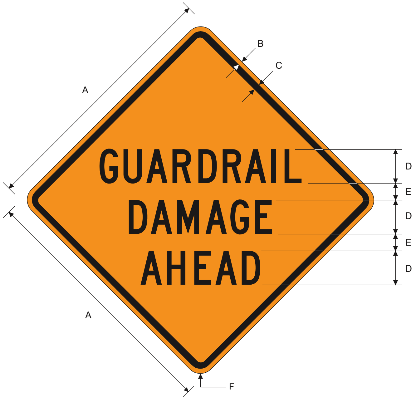
CW21-17T GUARDRAIL DAMAGE AHEAD
