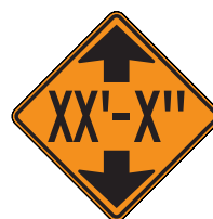
CW12-2 Clearance Advance
