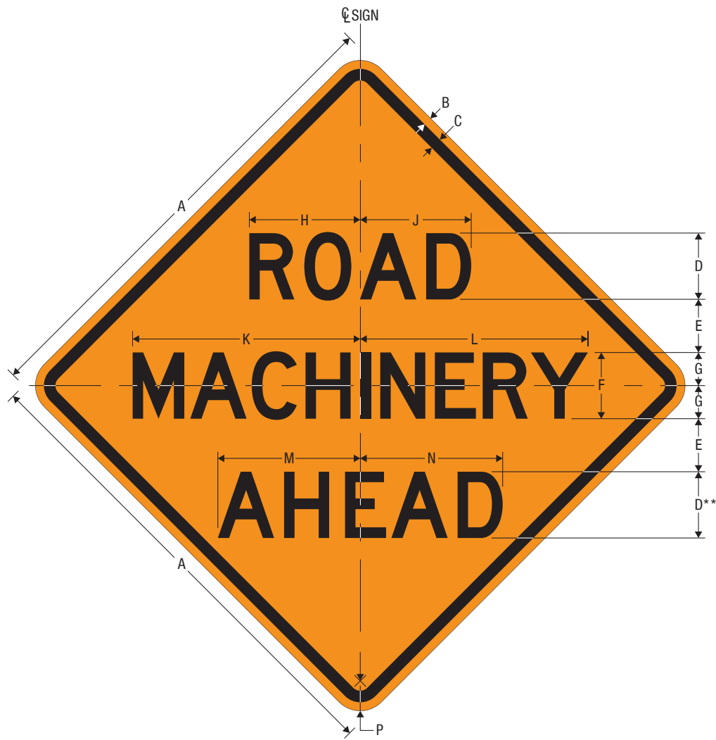
CW21-3[D] ROAD MACHINERY AHEAD
