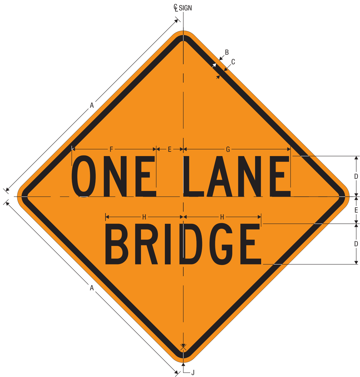
CW5-3 ONE LANE BRIDGE
