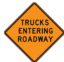
CW27-1T TRUCKS ENTERING ROADWAY
