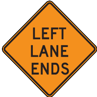
CW9-1L LEFT LANE ENDS
