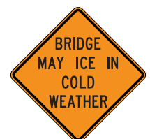
CW8-13aT BRIDGE MAY ICE IN COLD WEATHER
