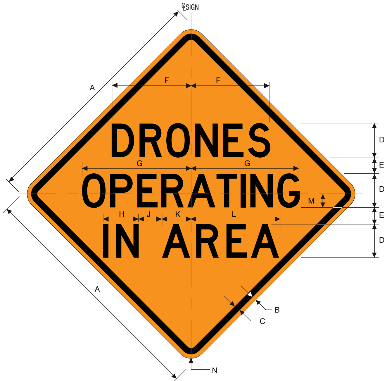
CW21-8T DRONES OPERATING IN AREA
