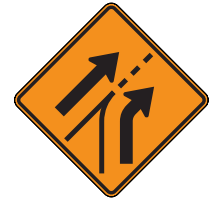
CW4-6R Entering Roadway Added Lane
