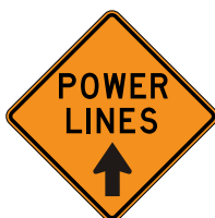
CW28-1T POWER LINES (with Arrow)
