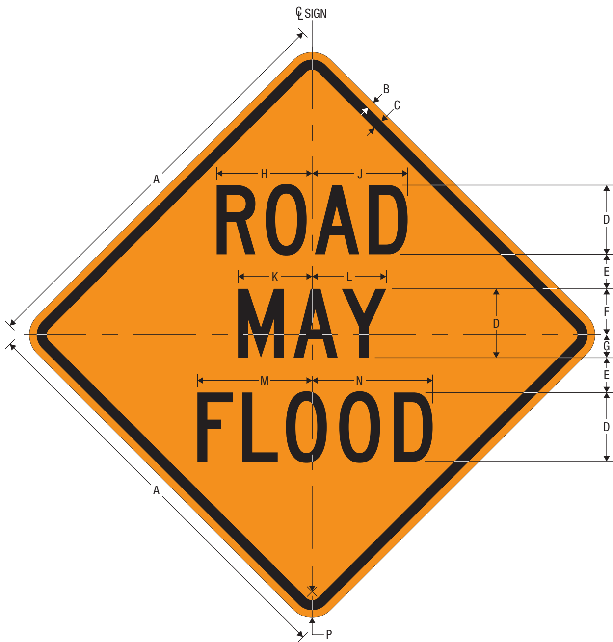
CW8-18 ROAD MAY FLOOD
