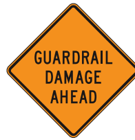
CW21-17T GUARDRAIL DAMAGE AHEAD
