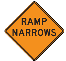
CW5-4 RAMP NARROWS
