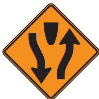
CW6-1 Divided Highway
