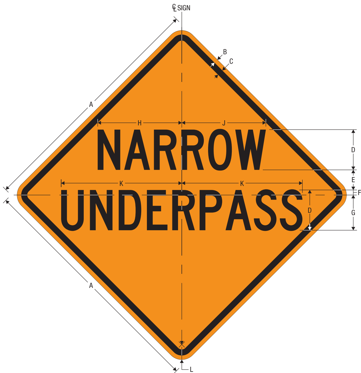
CW5-2a NARROW UNDERPASS
