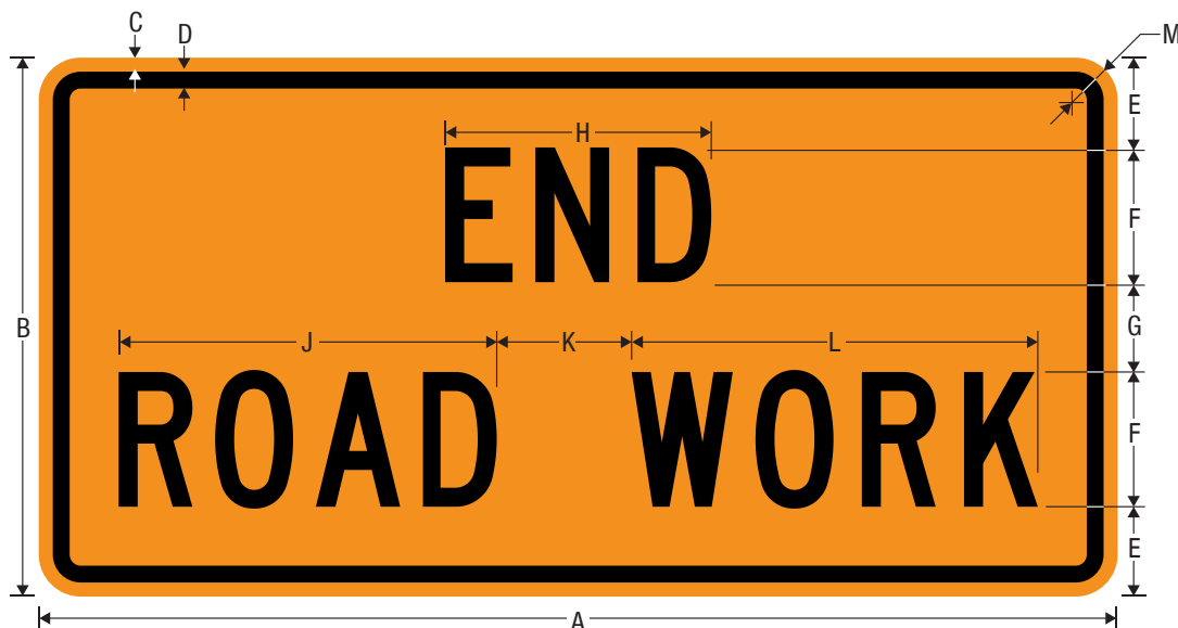
G20-2 END ROAD WORK
