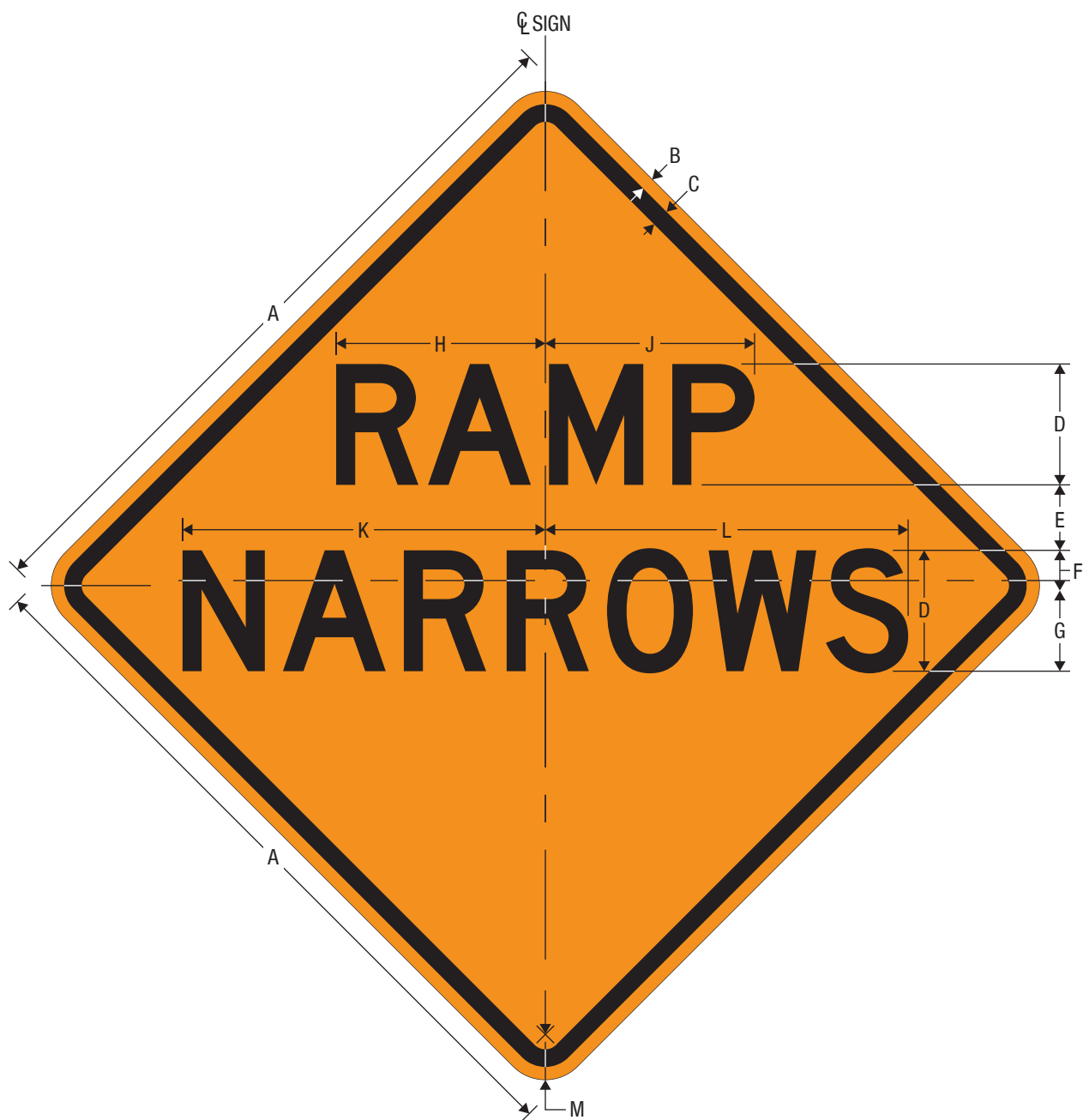
CW5-4 RAMP NARROWS
