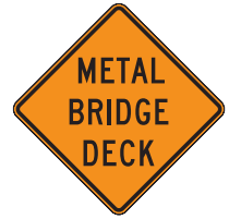
CW8-16 METAL BRIDGE DECK
