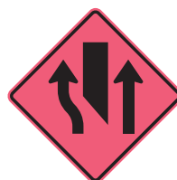
IMW9-3 Interior Lane Shift Ahead
