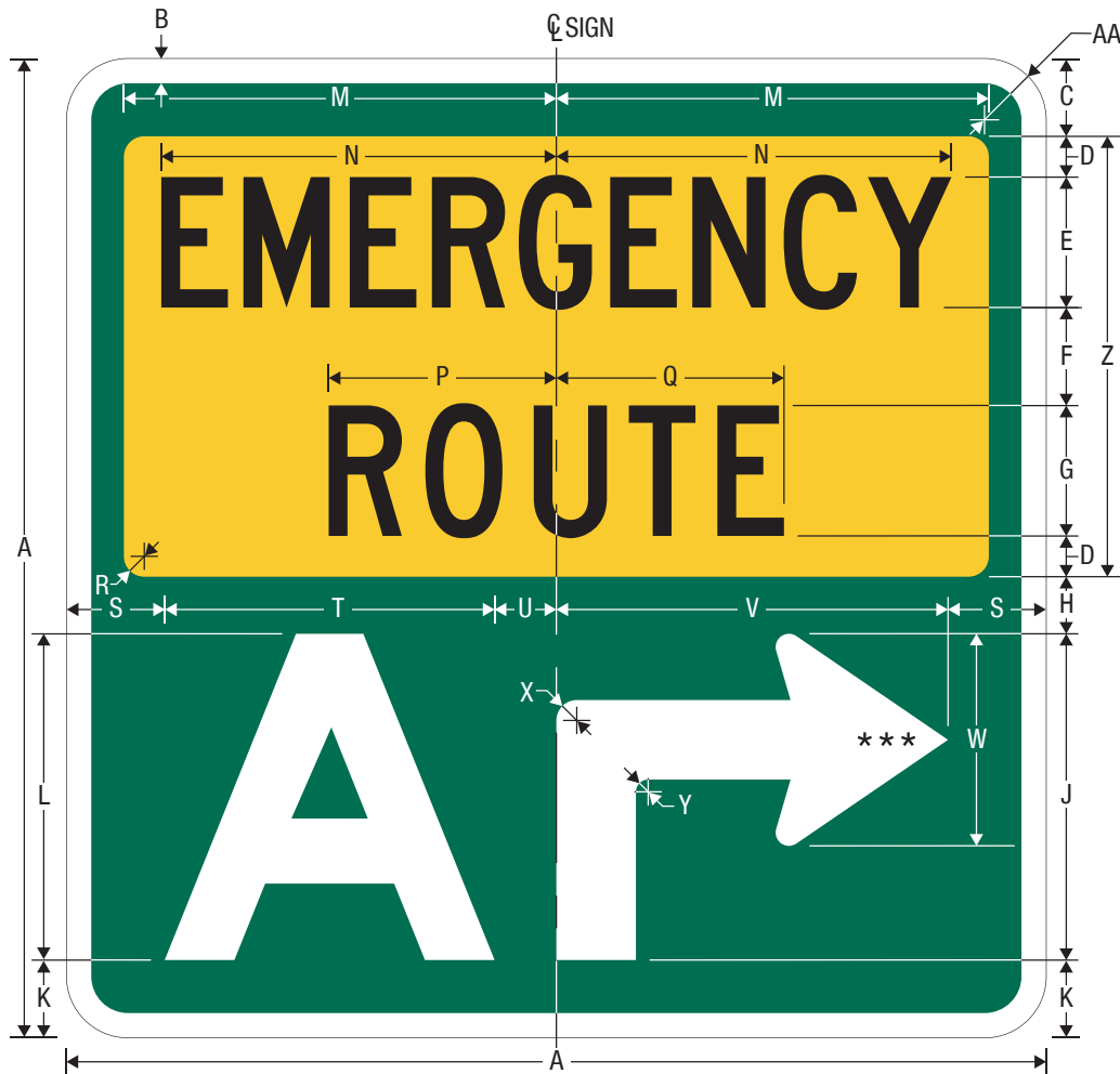
M4-11a[A]R EMERGENCY ROUTE Alternate (Right-Turn Arrow)
