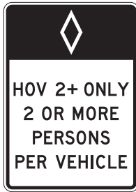
R3-10 Preferential Lane Vehicle Occupancy Definition (Post-Mounted)
