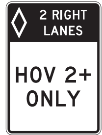
R3-11c Preferential Lane Operation - High- Occupancy Vehicles, Full-Time (Post-Mounted)
