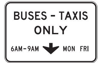
R3-14c Preferential Lane Operation (Overhead)
