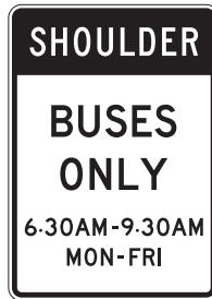
R3-11f Preferential Lane Operation (Post-Mounted)
