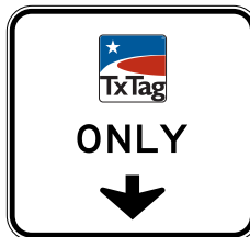
R3-44 Priced Managed Lane Operation (Overhead)
