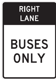
R3-11e Preferential Lane Operation - Full-Time (Post-Mounted)
