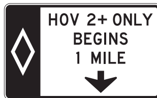
R3-15a HOV Lane Begins XX Miles (Overhead)
