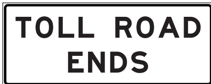
R90-3T TOLL ROAD ENDS
