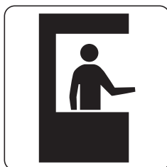
M4-17 Toll Collector Symbol Panel
