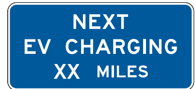
D9-17a NEXT EV CHARGING XX MILES
