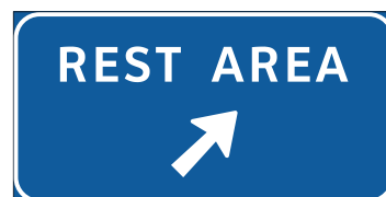
D5-2 REST AREA Entrance Direction
