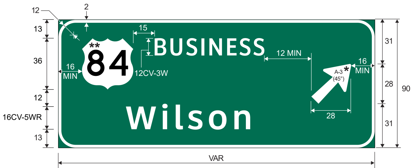
E4-2[B]b Exit Direction (1 Destination with Shield, Business)
