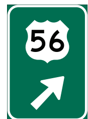
E4-1[D] Exit Direction (1 Shield) - Post-Mounted
