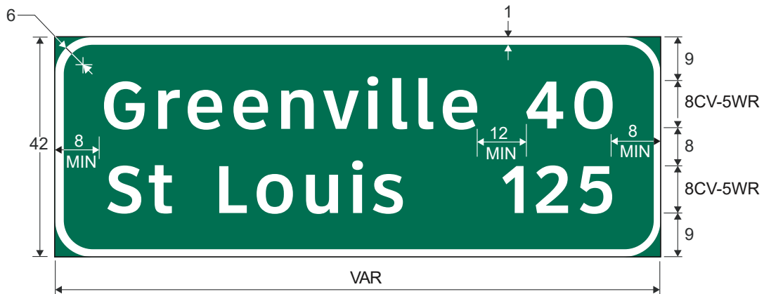
E7-2 (2 Lines) Post-Interchange Distance
