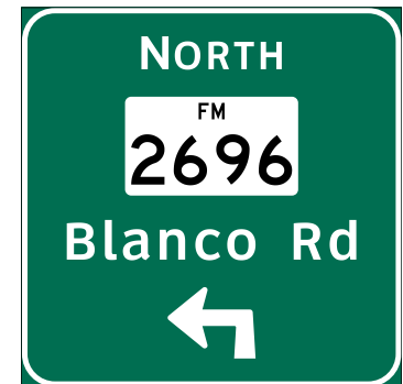
D1-7[A] Intersection Advance (with 90 Degree Left Arrow)
