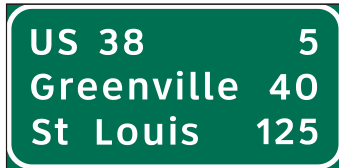
E7-3 (3 Lines) Post-Interchange Distance
