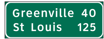
E7-2 (2 Lines) Post-Interchange Distance
