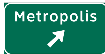
E4-1[C] Exit Direction (1 Destination) - Post-Mounted
