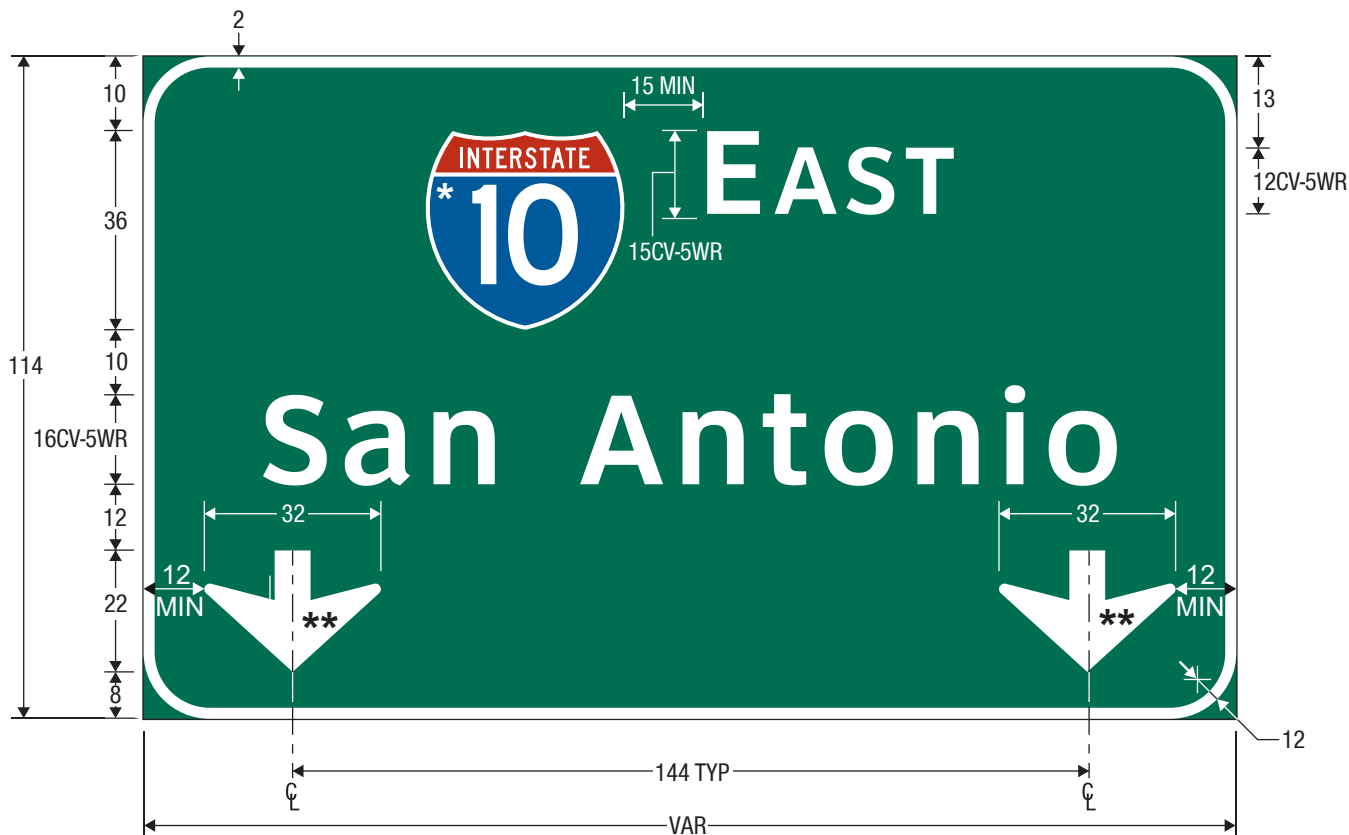
E6-2a Pull-Through (Destination, Down Arrows)
