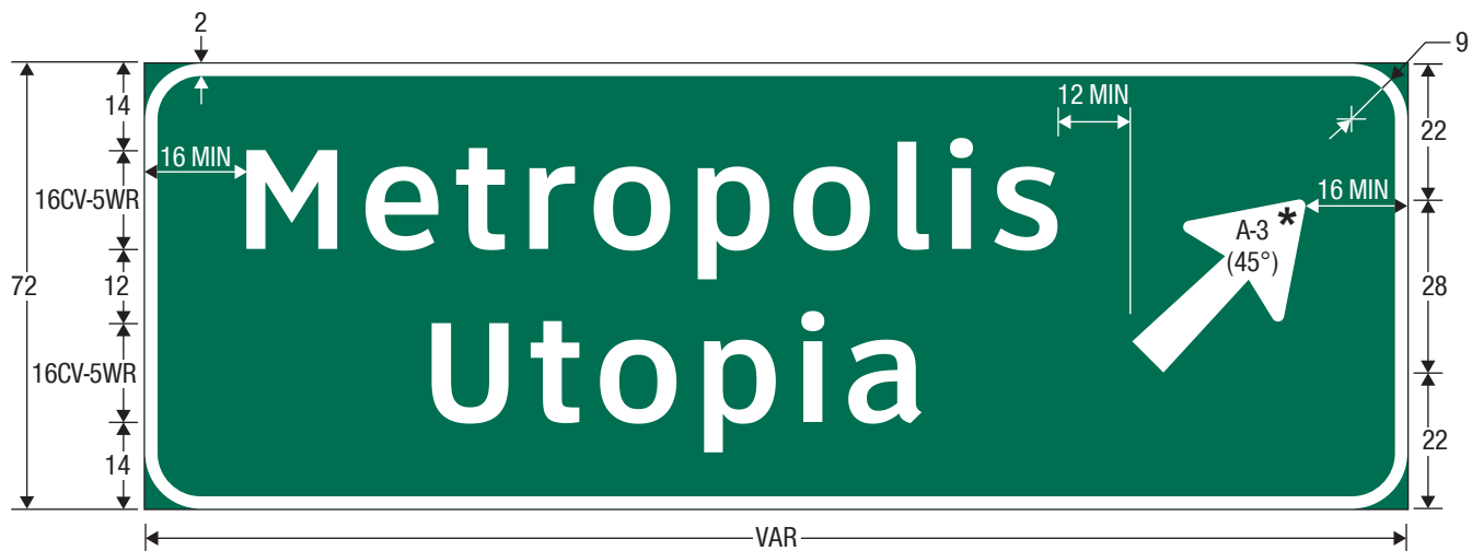
E4-2[A] Exit Direction (2 Destinations) - Overhead
