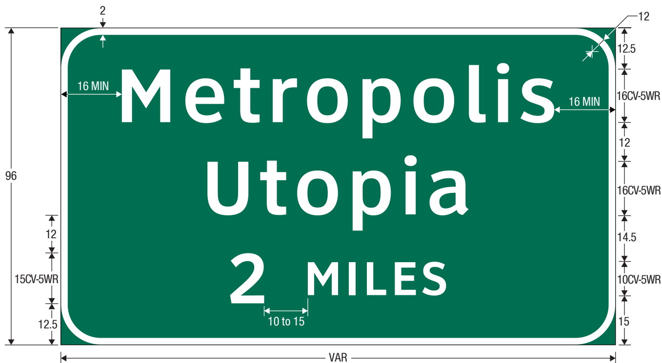
E1-2[A] Interchange Advance Guide (2 Destinations)
