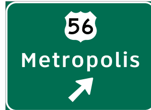
E4-2[D] Exit Direction (1 Destination with Shield) - Post-Mounted
