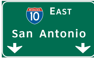
E6-2a Pull-Through (Destination, Down Arrows)
