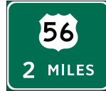
E1-1[B] Interchange Advance Guide (1 Shield)
