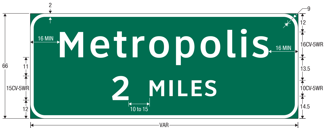
E1-1[A] Interchange Advance Guide (1 Destination)
