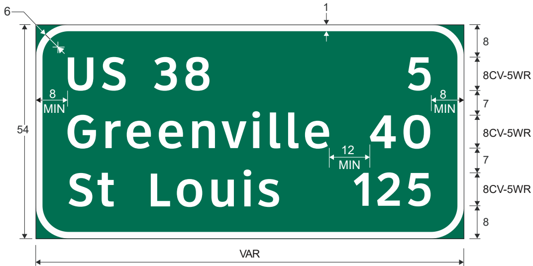
E7-3 (3 Lines) Post-Interchange Distance
