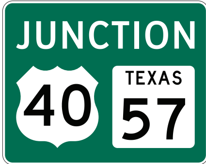
M2-2 Combination Junction (2 Route Signs)
