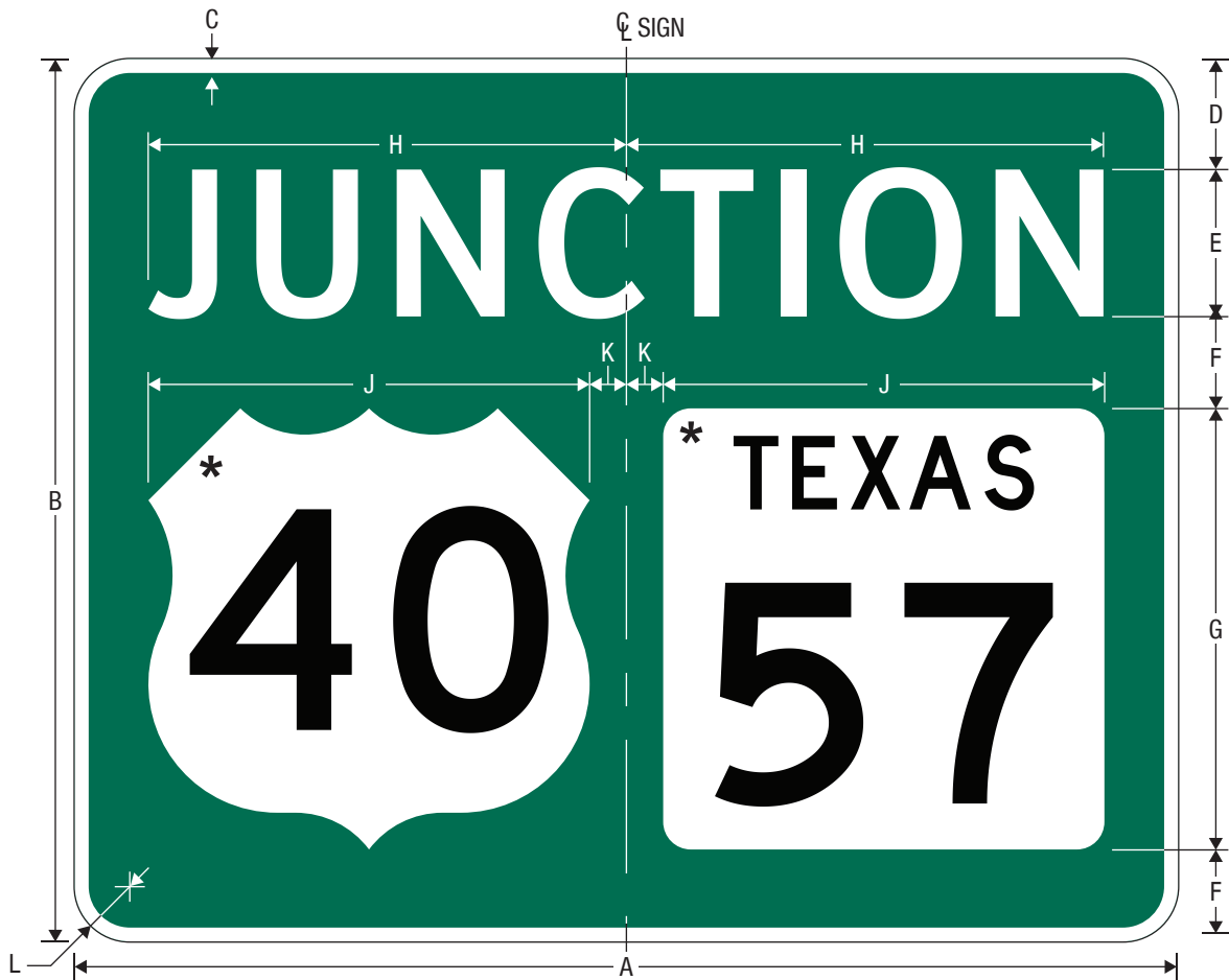
M2-2 Combination Junction (2 Route Signs)
