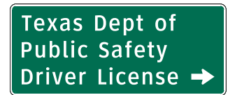
D26-2TR TEXAS DEPARTMENT OF PUBLIC SAFETY DRIVER LICENSE (Arrow)
