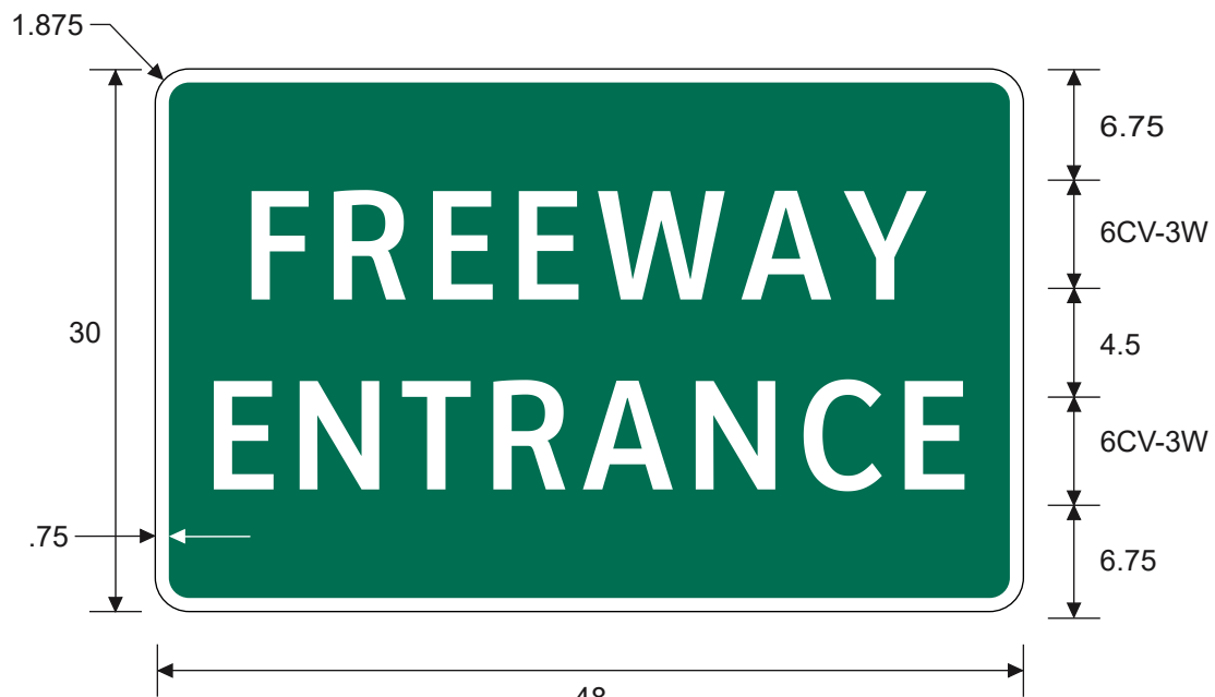
D13-3 FREEWAY ENTRANCE
