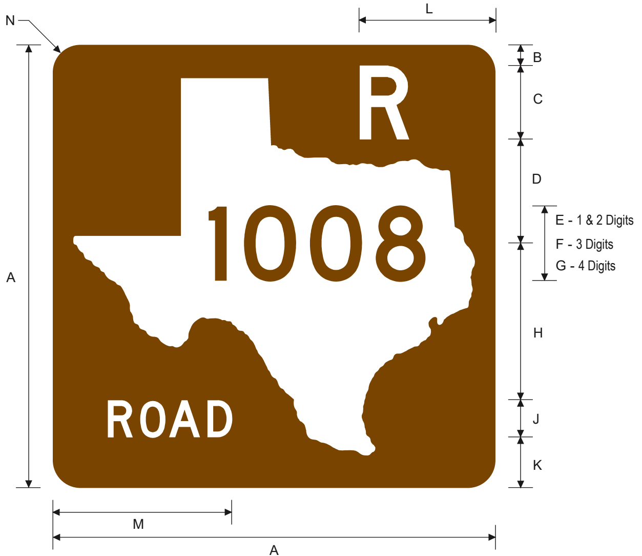
M1-5RR RR Road Route Marker (Independent)
