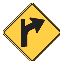
W1-10bR Combination Horizontal Alignment/ Intersection
