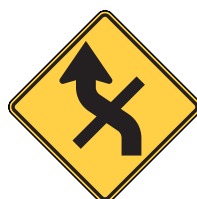
W1-10eL Combination Horizontal Alignment/ Intersection
