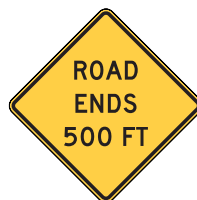
W8-26 ROAD ENDS Advance
