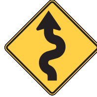
W1-5L Horizontal Alignment - Winding Road
