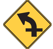
W1-10aL Combination Horizontal Alignment/ Intersection
