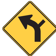
W1-10L Combination Horizontal Alignment/ Intersection
