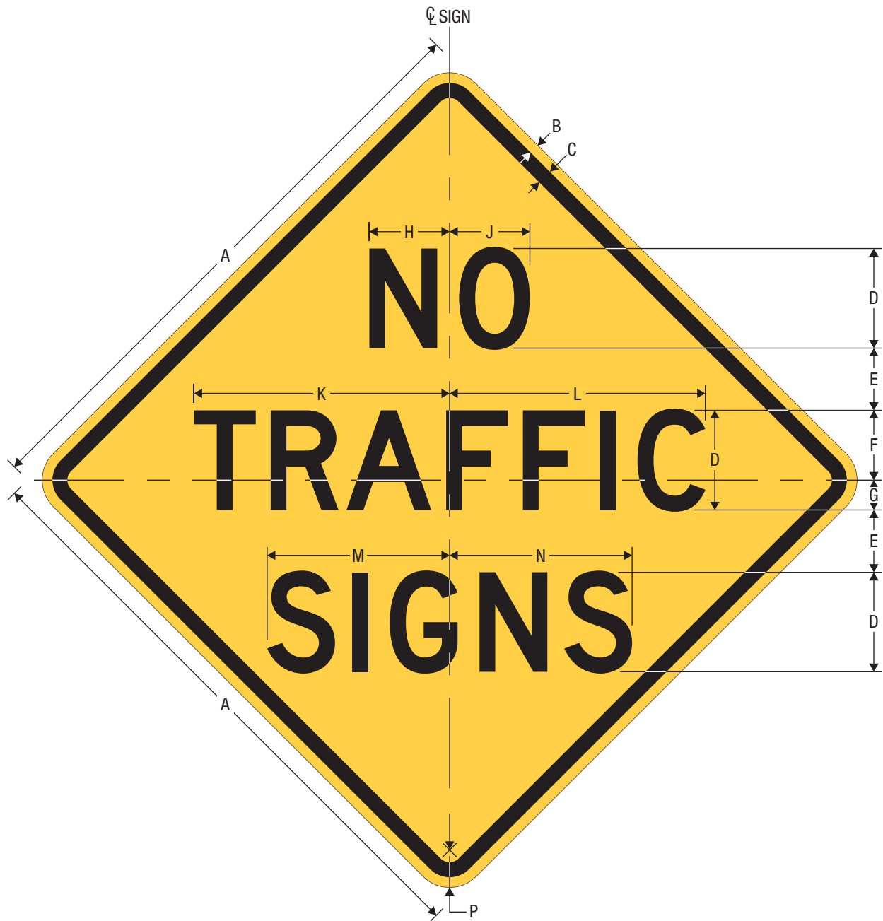
W18-1 NO TRAFFIC SIGNS
