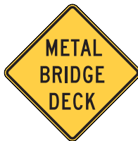
W8-16 METAL BRIDGE DECK
