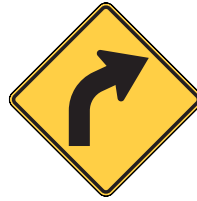
W1-2R Horizontal Alignment - Curve
