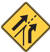
W4-6R Entering Roadway Added Lane
