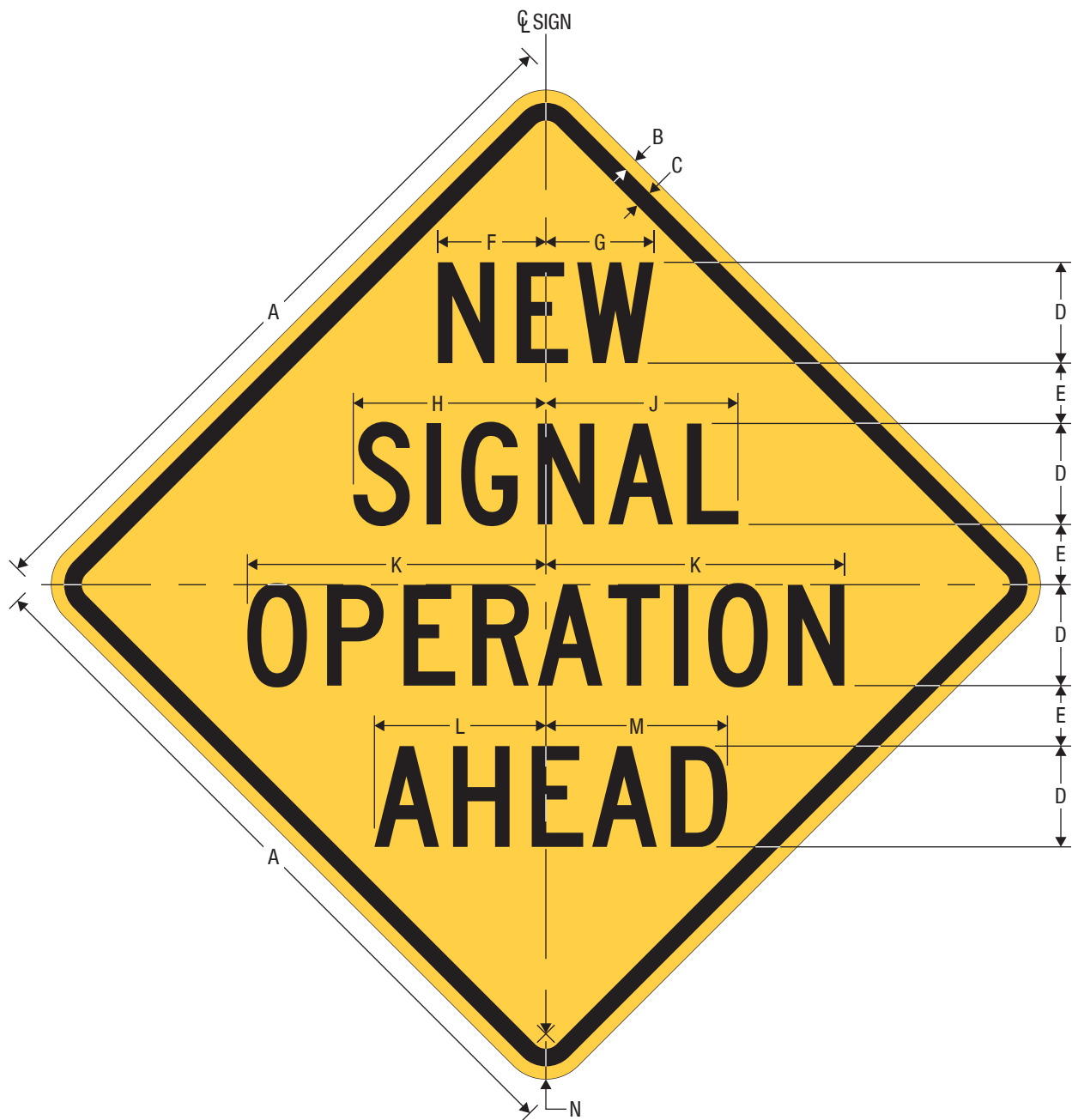
W23-2a NEW SIGNAL OPERATION AHEAD
