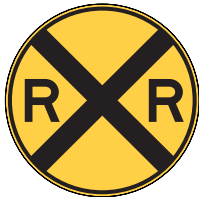
W10-1 Grade Crossing Advance Warning
