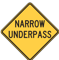
W5-2a NARROW UNDERPASS
