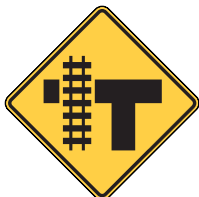
W10-4L Grade Crossing Advance Warning - T-Intersection with Grade Crossing
