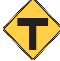
W2-4 Intersection Warning - T-Intersection
