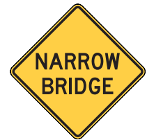
W5-2 NARROW BRIDGE
