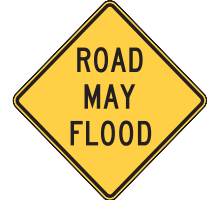
W8-18 ROAD MAY FLOOD
