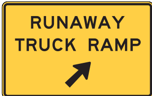
W7-4b RUNAWAY TRUCK RAMP Entrance Direction
