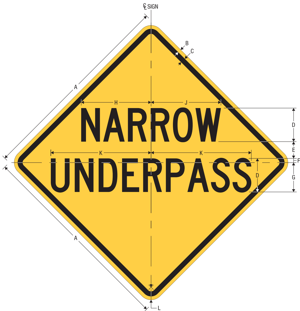
W5-2a NARROW UNDERPASS
