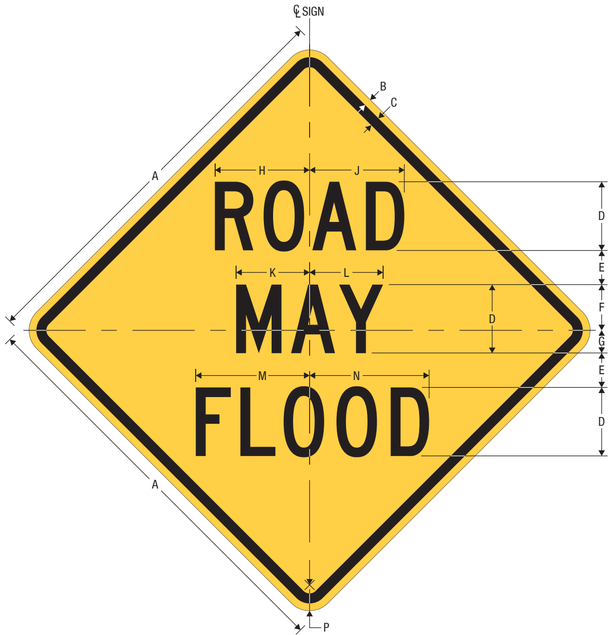
W8-18 ROAD MAY FLOOD
