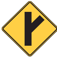
W2-3R, W2-3aL Intersection Warning - Oblique Side Road
