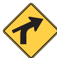
W1-10cR Combination Horizontal Alignment/ Intersection
