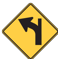
W1-10bL Combination Horizontal Alignment/ Intersection
