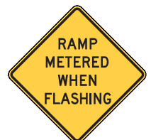
W3-8 RAMP METERED WHEN FLASHING
