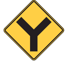
W2-5 Intersection Warning - Y-Intersection
