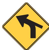
W1-10cL Combination Horizontal Alignment/ Intersection
