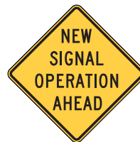
W23-2a NEW SIGNAL OPERATION AHEAD
