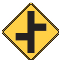
W2-7L Intersection Warning - Offset Side Roads
