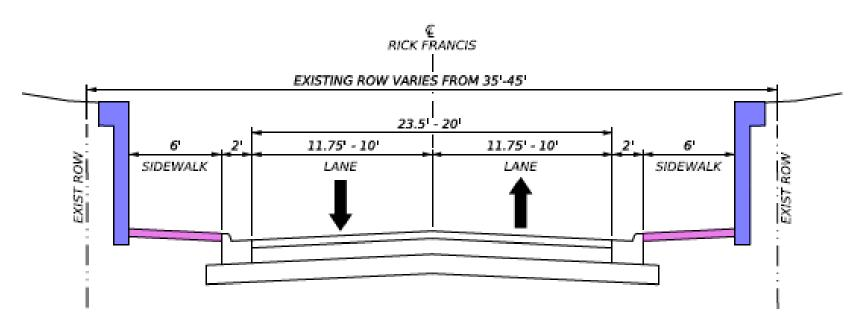
UNDERPASS CONCEPT RETAINING WALL SECTION TWO-LANE
