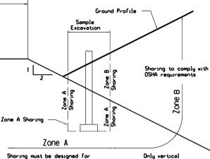
Shoring must be designed for Railroad live load surcharge in addition to OSHA Standard loads for excavation in Zone A.
