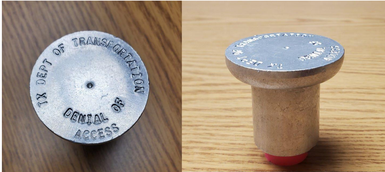
Figure 6 Example Denial of Access Marker. NIGP 30578532100. Marker, survey, denial of access, 2-inch alum for 5/8-inch rebar.
