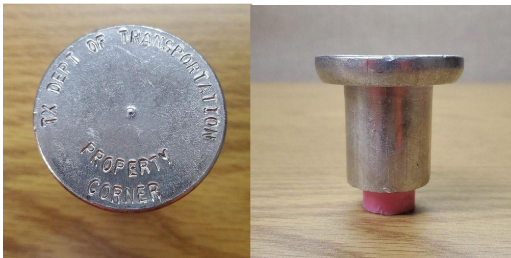
Figure 5 Example Property Corner Marker. NIGP 30578532209. Marker, survey, property corner, 2-inch alum cap for 5/8-inch rebar.
