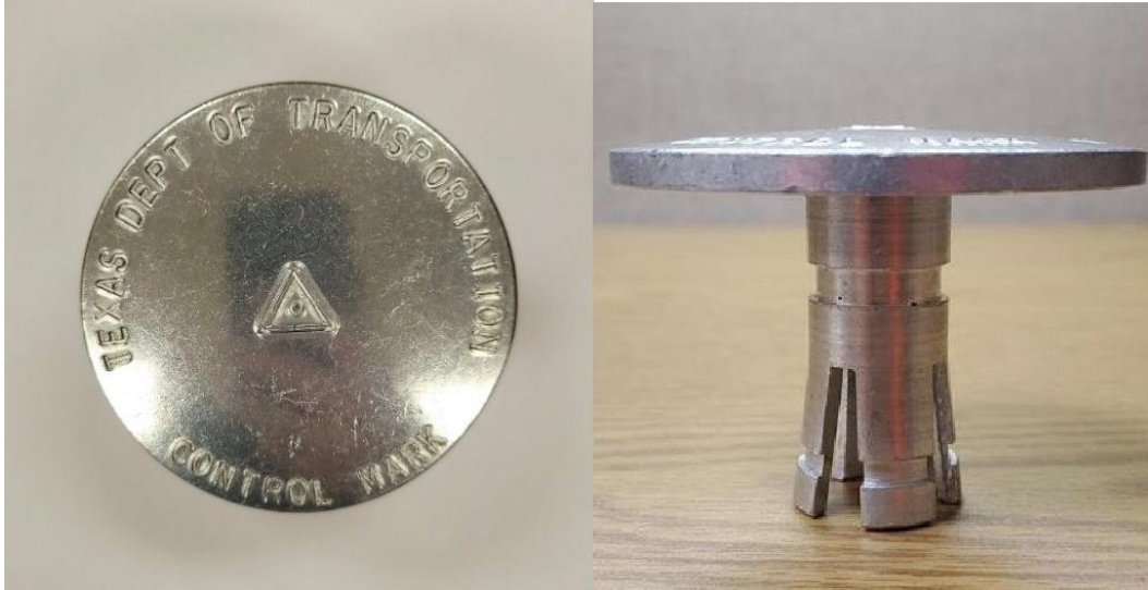
Figure 3 Example Control Point Marker. Profile view to set in concrete and set with 5/8-inch rebar. Configuration A: NIGP 30578532464. Marker, Survey, Control point, 3 ½-inch alum for rock and concrete. Configuration B: NIGP 30578532514. Marker, Survey, Control point, 3 ¼-inch alum rebar cap.
