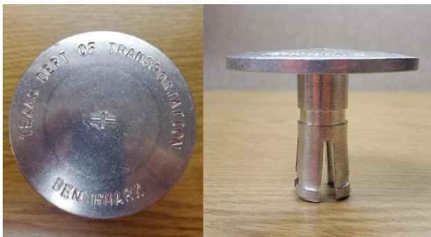
Figure 4 Example Benchmark Marker. Profile view to set in concrete and set with 5/8-inch rebar. Configuration A: NIGP 30578532472. Marker, Survey, Benchmark, 3 ½-inch alum for rock or concrete. Configuration B: NIGP 30578532506. Marker, Survey, Benchmark, 3 ¼-inch alum cap for 5/8-inch rebar.
