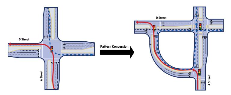
FIGURE 7 - TRADITIONAL INTERSECTION (LEFT) / QUADRANT ROADWAY (RIGHT) COMPARISON
