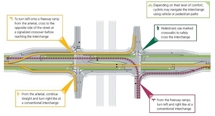
FIGURE 3 - DISPLACED LEFT TURN INTERCHANGE
