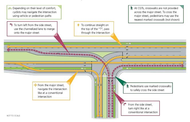
FIGURE 2 - CGT INTERSECTION (THREE-LEGGED DESIGN)
