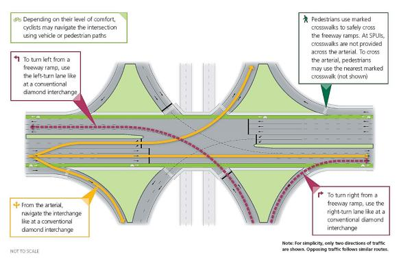
FIGURE 9 - SINGLE POINT URBAN INTERCHANGE (SPUI)
