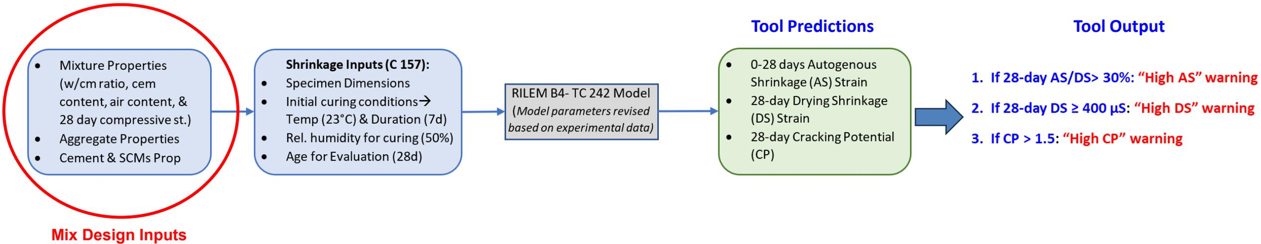
1. Autogenous Shrinkage (AS) Evaluation → sealed concrete prisms, mod. ASTM C 1698 (only for se
