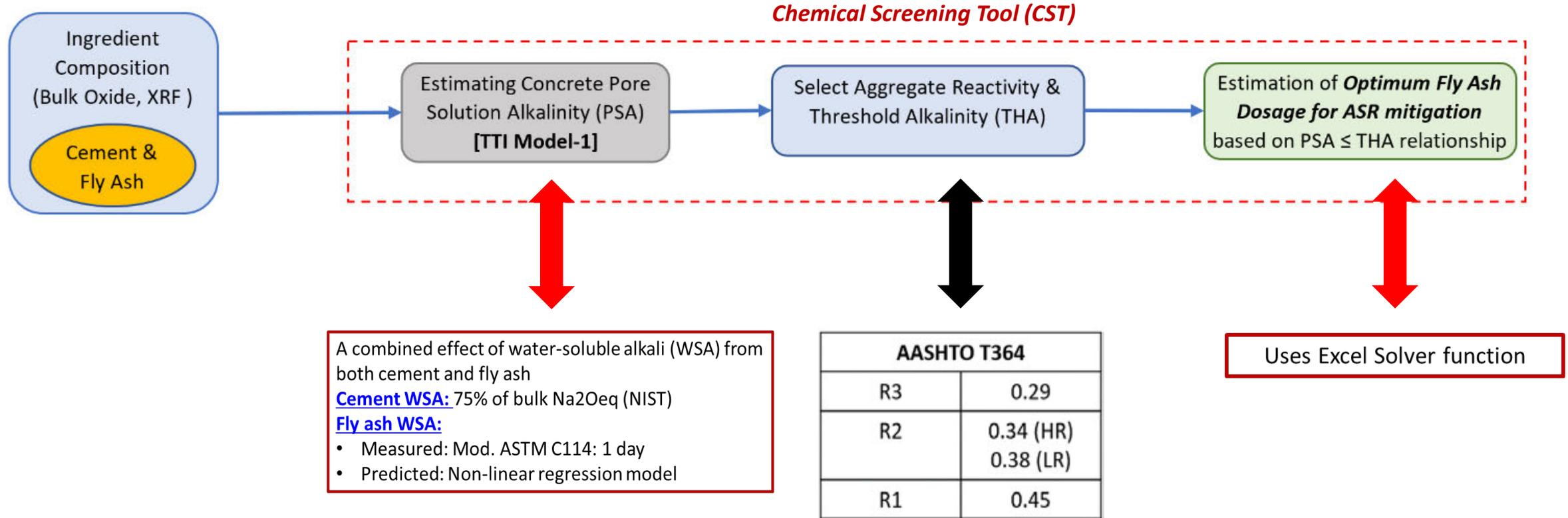
1. Saraswatula, P., Mukhopadhyay, A., & Liu, K. W. (2022). Development of a Screening Tool for Rapid Fly Ash Evaluation for Mitigating Alkali Silica Reaction in Concrete. *Transportation Research Record*
