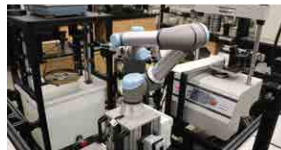
The AMAZE can automatically perform four asphalt mixture tests. Photo by Martin Dassi
