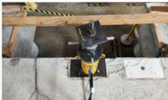
(c) Punching shear failure from top
