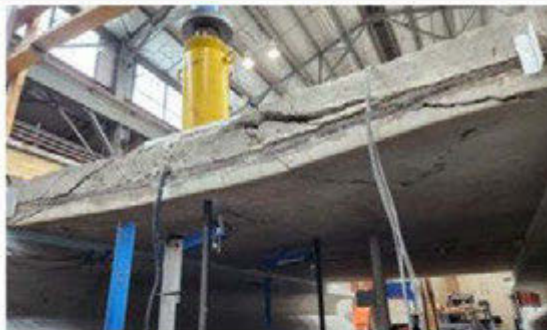
(b) Punching shear failure from bottom
