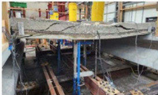
(a) Punching shear failure from side
