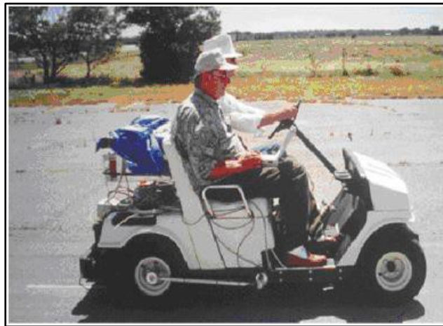
Figure 2 —Illustration of a Lightweight Inertial Profiler Developed by the Department
