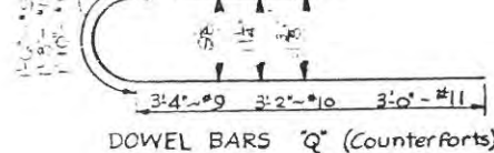
DOWEL BARS "Q" (Counterforts)
