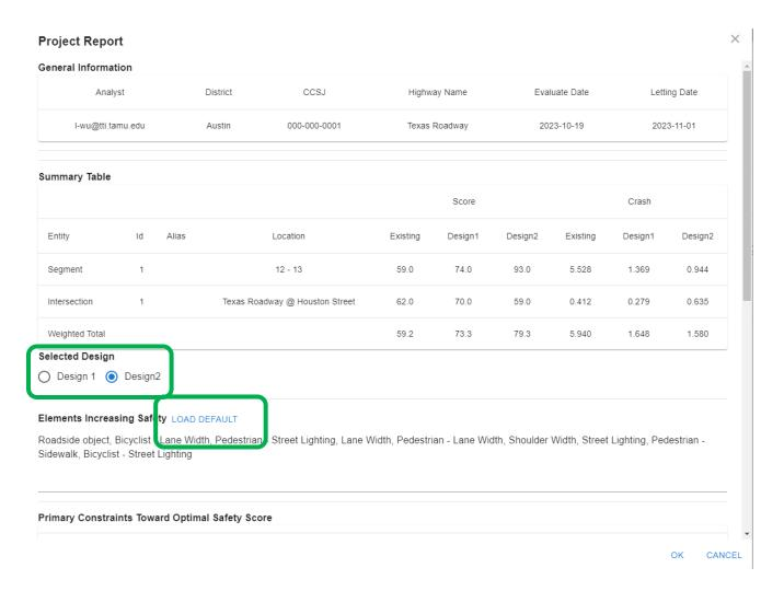
For elements increasing safety, the "LOAD DEFAULT" button will compare the selected design (i.e., Design1 or Design2) with existing configurations, and fill the report by comparison results. This feature is provided to make the assessment process easier, users are encouraged to verify the default values, and should be modified when needed.
