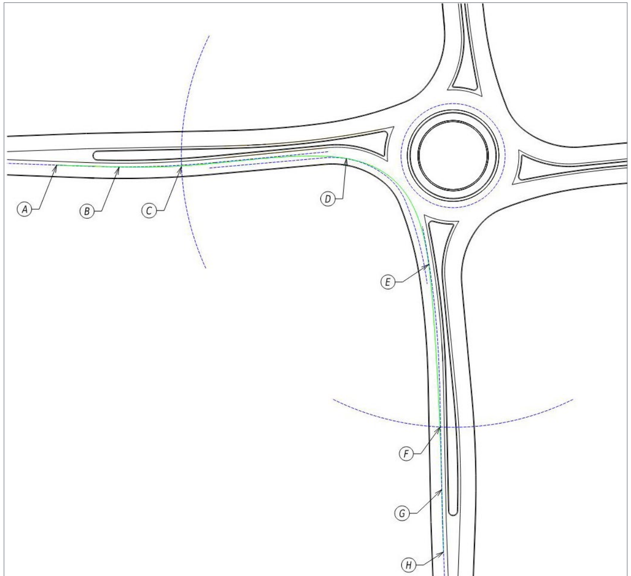
» FIGURE 10 – Typical Point Placement on a Right-Turn Spline
