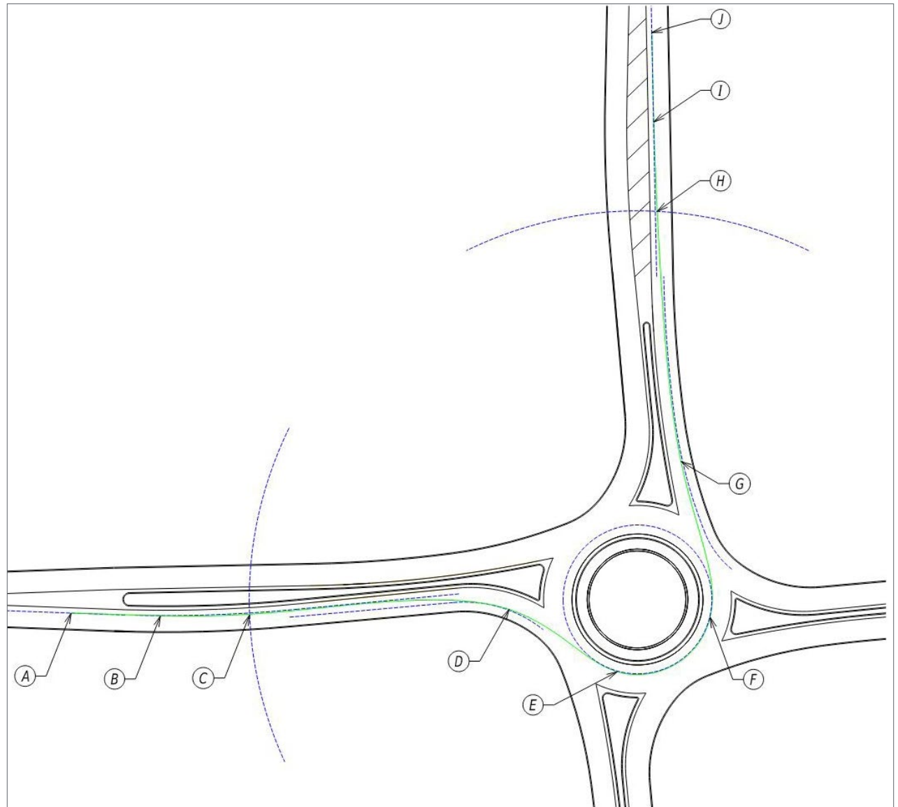
» FIGURE 9 – Typical Point Placement on a Left-Turn Spline
