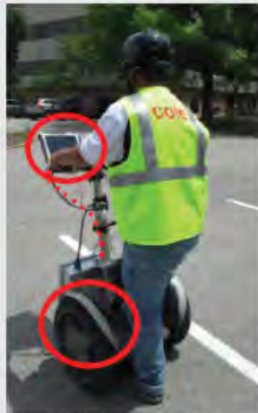
The ULIP-ADA is pictured highlighting the ULIP box and the laptop, which synchs the device to GIS.
