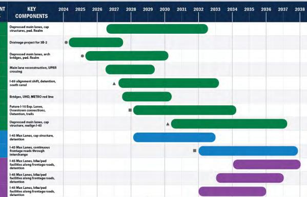
3B-1 is phased to start before 3B-2 because drainage elements in 3B-1 need to be constructed and operational to receive drainage from 3B-2.
