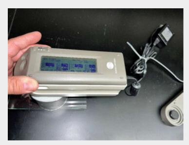
TEX-823-B: Color Measurement of Glass Beads Federal Test Method Standard 141, Method 4252.
