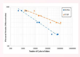
Fig. 2. Estimated Life until Failure
