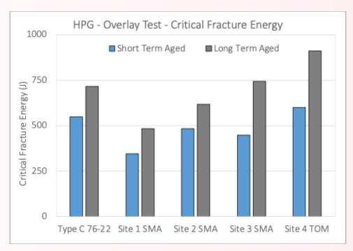
**Overlay Cracking Test Results**
