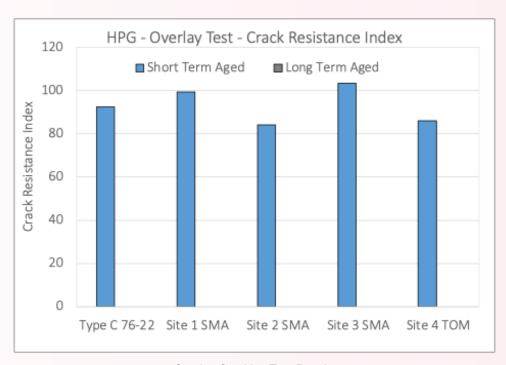
**Overlay Cracking Test Results**
