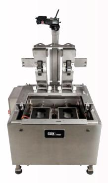
Hamburg Wheel-Tracking Test Setup
