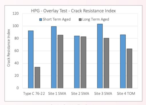
**Overlay Cracking Test Results**
